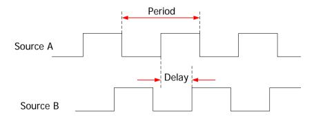
Source A and source B can be CH1 or CH2.
