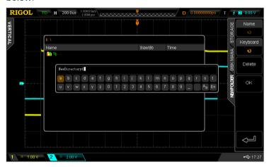
This oscilloscope supports Chinese/English input method. The file name or folder name can contain letters, numbers, underscores, spaces and Chinese characters and the length of the characters is limited to 64 bytes. The following part introduces how to input a file name or folder name using Chinese/English input method.
