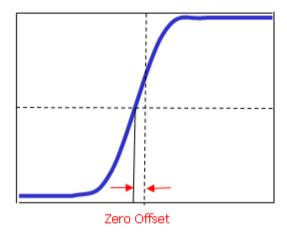
Press CH1 → Delay-Cal and use ♦ to set the desired delay time. The range available is from -100 ns to 100 ns.
