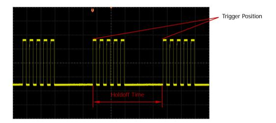
Press MENU → Setting → Holdoff in the trigger control area (TRIGGER) at the front panel and use ♦ to modify the holdoff time (the default is 100 ns) until the waveform triggers stably. The adjustable range of holdoff time is from 100 ns to 10 s. Note that trigger holdoff is not available for Nth edge trigger, video trigger, RS232 trigger, I2C trigger, SPI trigger and USB trigger.
