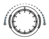
This knob provides quick Adjust/Locate function for numerical parameters with relatively larger settable range. Turn clockwise (counterclockwise) to increase (reduce) the value. The inner knob is used for fine adjustment and the outer knob for coarse adjustment.
