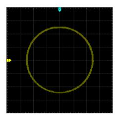
4. As shown in the figure above, the distances from the crossing points of axis and the circle to the origin of the coordinates are approximately equal. Thus, the phase deviation angle θ=±arcsin1=90°.
