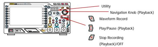
Press Utility → Record → Mode and use ♦ to select "Record" to open the waveform record operation menu.
