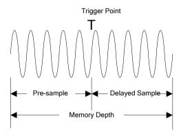
The relation of memory depth, sample rate and waveform length fulfills the equation below:
