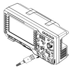
Figure 1-5 To Connect the Probe
