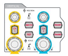
ch1, ch2: analog input channels. The 2 channels are marked by different colors which are also used to mark both the corresponding waveforms on the screen and the channel input connectors. Press any key to open the corresponding channel menu and press again to turn off the channel.
