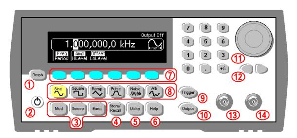
Lighted keys indicate active keys and functions (for example Sine above).
