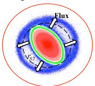
Diocotron modes are ExB-drift surface waves on magnetized electron plasma columns, and are isomorphic to Kelvin waves on vortices in 2D Euler flows. The image at left shows the measured vorticity (colors) in a large  $m_{\theta}$ =2 (elliptical) wave. *Exponential* Landau damping (inviscid vortex symmetrization) occurs when vorticity interacts with the wave at the resonant radius  $r_{s2}$ , typically ceasing when a nonlinear "cat's eye" structure (blue) forms.
