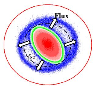
Diocotron modes are  $\mathbf{E} \times \mathbf{B}$ -drift surface waves on magnetized electron plasma columns, and are isomorphic to Kelvin waves on vortices in 2D Euler flows. The image at left shows the measured vorticity (colors) in a large  $m_{\theta} = 2$  (elliptical) wave. *Exponential* Landau damping (inviscid vortex symmetrization) occurs when vorticity interacts with the wave at the resonant radius  $r_{S2}$ , typically ceasing when a nonlinear "cat's eye" structure (blue) forms.
