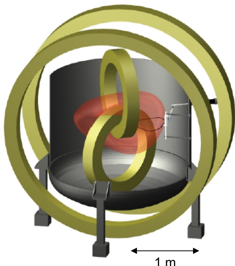
FIG. 15 (color online). The Columbia non-neutral torus (CNT) showing a cutaway of the vacuum vessel, the four circular magnetic field coils used to produce the stellerator field, and the calculated magnetic surfaces (faint deformed donut). From T. S. Pedersen.
