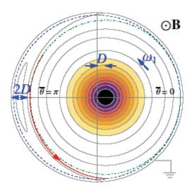
**FIGURE 1.** Instantaneous cross section of an electron plasma column in the diocotron displacement  $\vec{D}$ . The black-to-orange filled region is the dense plasma core. The gray lines are the equipotential contours in the mode frame. The green dotted-dashed curve is resonance contour. The red solid curve is a resonant particle trajectory. The blue dashed curve is the scrape-off layer.
