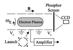
FIG. 2. Electron trap with CCD camera density diagnostic. The wall signal from sectored electrodes is used to measure the wave amplitudes.
