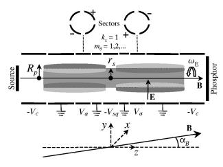
FIG. 1. Schematic of electron plasma with a trapped particle mode in the cylindrical containment system.
