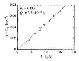
FIG. 3. Net growth rate vs ion current.
