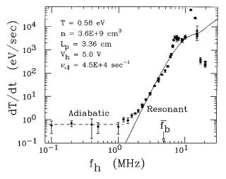
FIG. 2. Measured heating rates versus frequency of applied voltage. Adiabatic heating dominates at low  $f_h$ , while resonant heating dominates at high  $f_h$  (enhanced by damped-mode heating near 7 and 11 MHz). The dashed curve is from Eq. (1), and the solid curve is from Eq. (2), both with  $\delta L/L_p = 0.0042$ .
