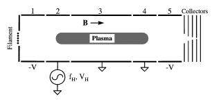
FIG. 1. Schematic of the cylindrical apparatus and electron plasma. Cylinders 2 and 4 are the same length.
