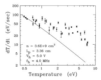
FIG. 5. Measured heating rate decreases slowly with plasma temperature. The solid curve shows the prediction of Eq. (2) with  $\delta L/L_p=0.0042$  and  $\overline{f_b}=6.22T({\rm eV})$  MHz.
